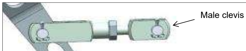
Figure 41-23: Adjust gap between tail valve pin and lever
