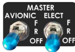
Figure 24-2: Master switch placard
