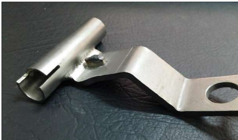
Figure 27-6: FH Lock block after weld
