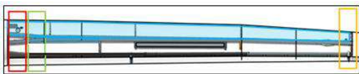
Figure 41-1: Main wing tanks (blue)
