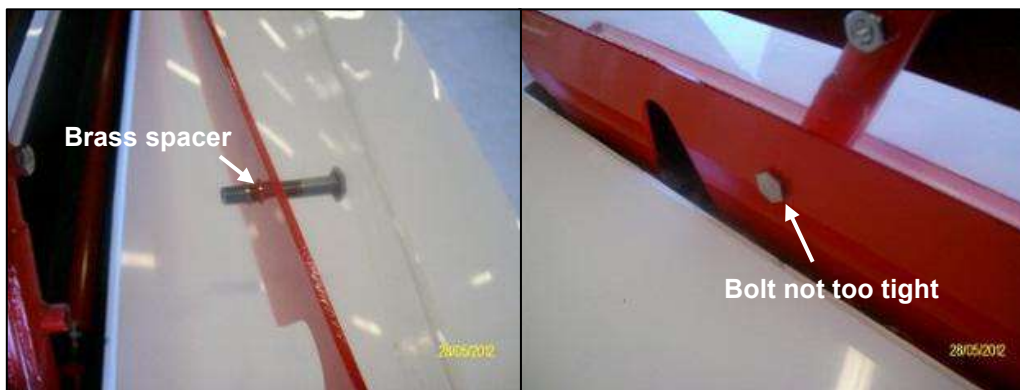
Figure 27-36: Brass spacer and bolt tightening
