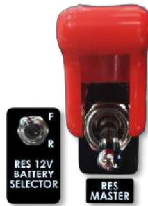
Figure 24-3: RES Master switch and battery selector
