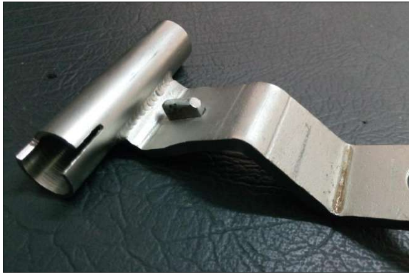
Figure 27-7: Example of correctly repaired FH lock block
