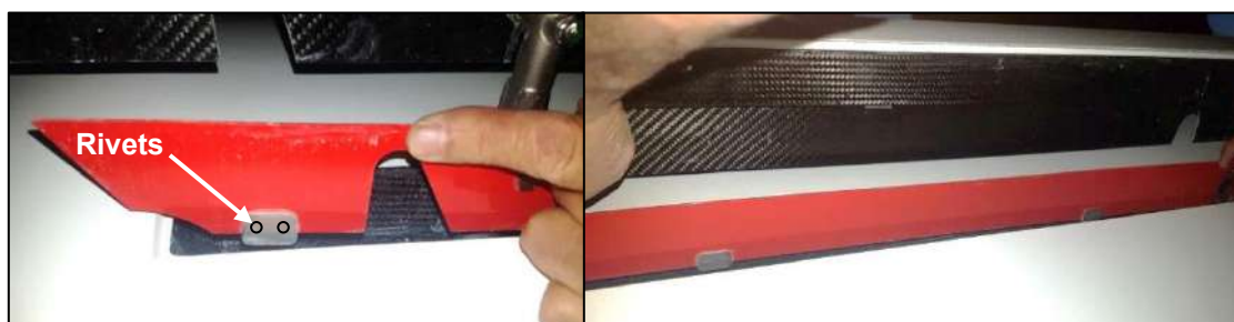
Figure 27-37: Metal tabs riveted onto airbrake blade 3
