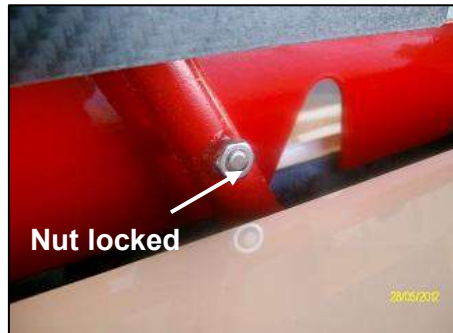
Figure 27-38: Bolt airbrake blade 3 onto airbrake lifters
