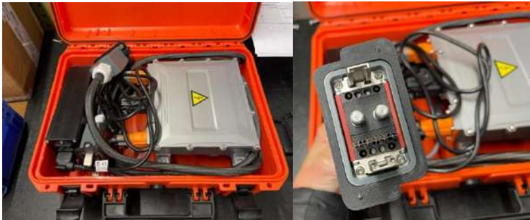
Figure 24 RES HV battery charger
