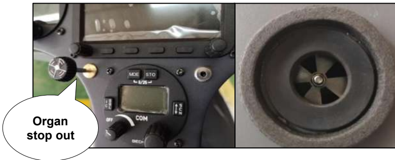
Figure 7-9: De-misting valve open
