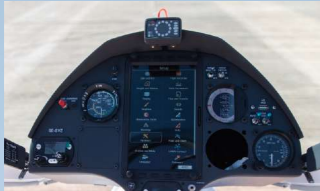
Flarm LED mounted in front of coaming
