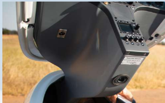
Male XLR Remote Battery Charging Socket Under Binnacle
