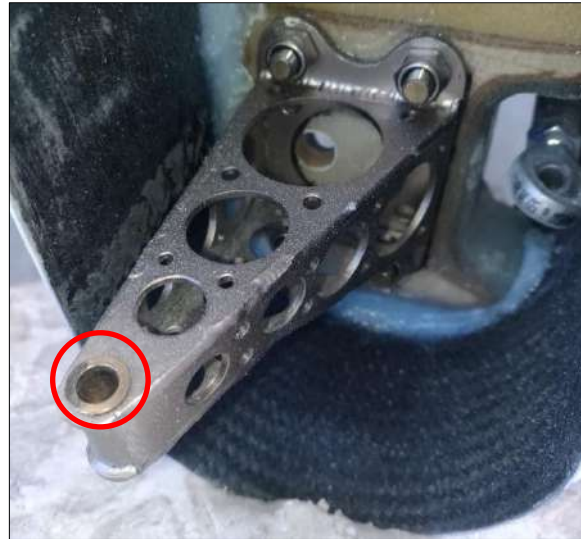
Figure 27-13: Brass bush removal
