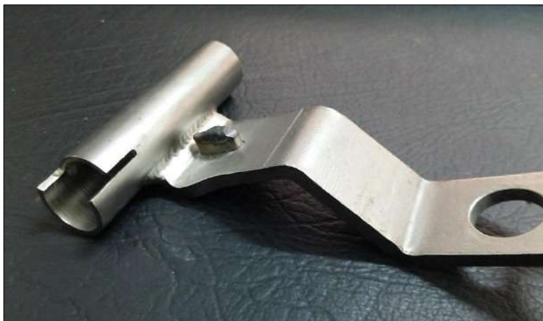
Figure 27-6: FH Lock block after weld
