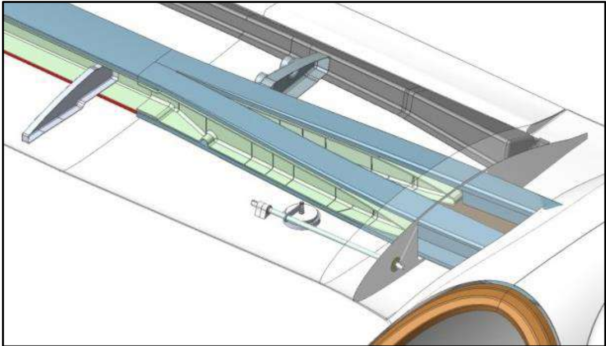
Figure 41-12: Main wing water valve
