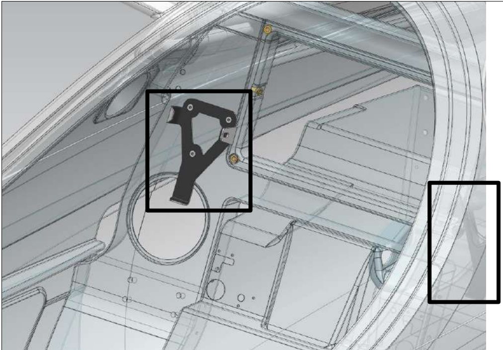
Figure 39-12: Bug wiper motor mounting brackets
