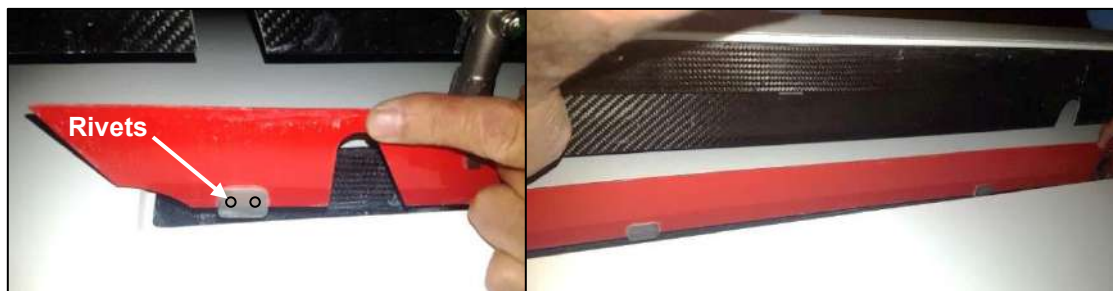
Figure 27-37: Metal tabs riveted onto airbrake blade 3
