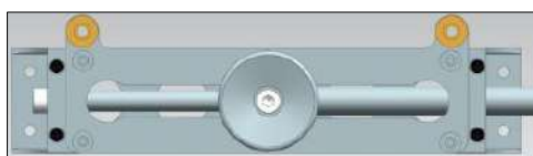
Figure 41-21: Water system lever in the centre position
