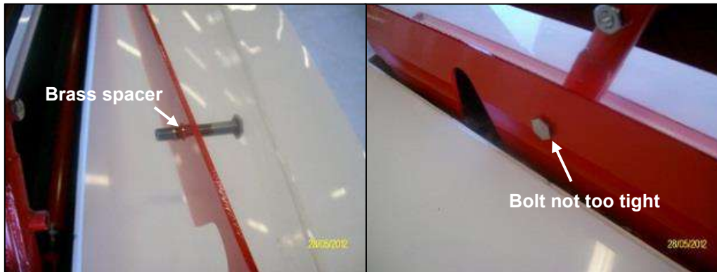
Figure 27-36: Brass spacer and bolt tightening
