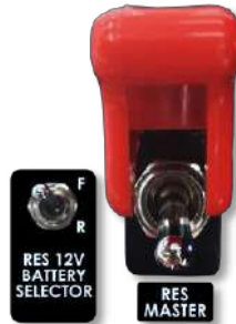
Figure 24-3: RES Master switch and battery selector
