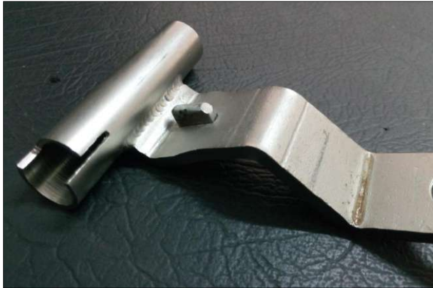
Figure 27-7: Example of correctly repaired FH lock block
