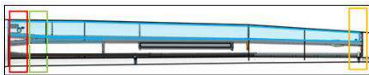
Figure 41-1: Main wing tanks (blue)
