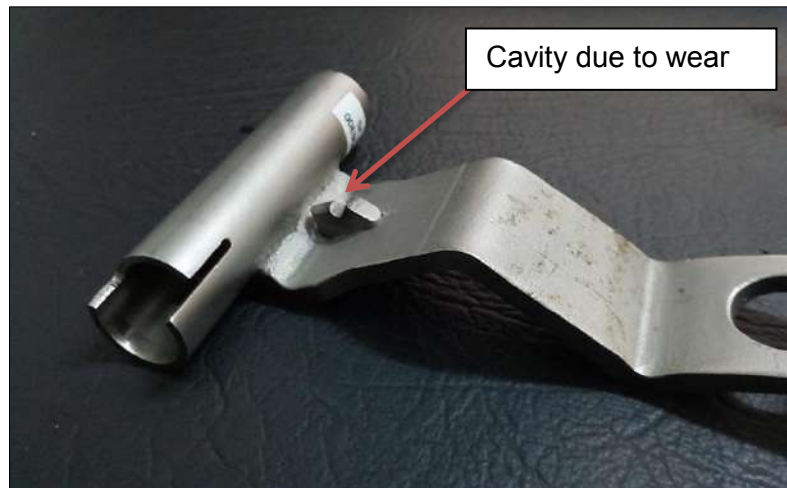
Figure 27-5: Wear on flap handle lock block
