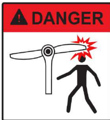
Figure 2-4 Propeller warning placard
