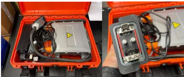
Figure 8-3 RES HV battery charger
