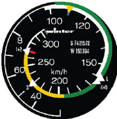
Figure 2-1 ASI in km/h
