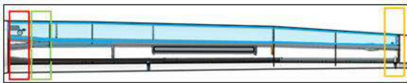
Figure 7-20: Main wing tanks (blue)
