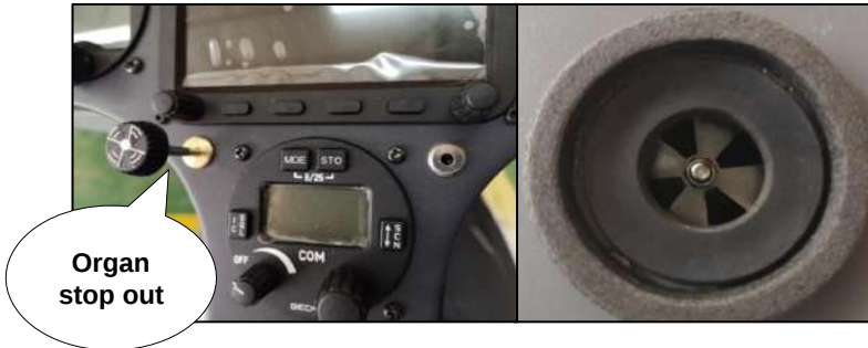
Figure 7-9: De-misting valve open
