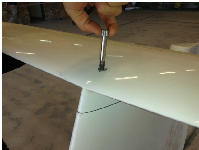
Fig. 1 - Loosening of Captive Bolt
