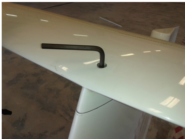
Fig. 1 - Loosening of Captive Bolt
