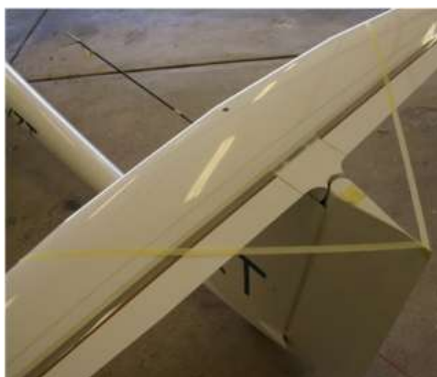
Figure 2: Centralise and Hold Rudder in Position with Masking Tape
