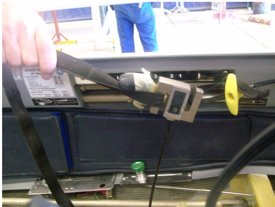
Figure 2 Example of load test setup using a load cell
