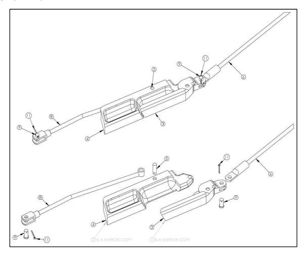
If either split pin is missing, or appears to be slipping out, replace it immediately.
