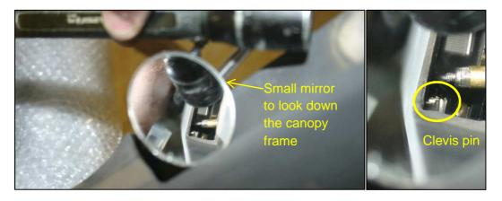
Both Clevis pins (Item 9) must be installed from below and each must be secured by a split pin (Item 11).
