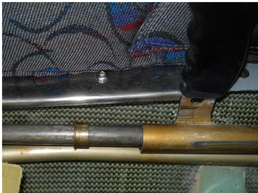
Figure 1: Landing gear handle with unseated brass bush
